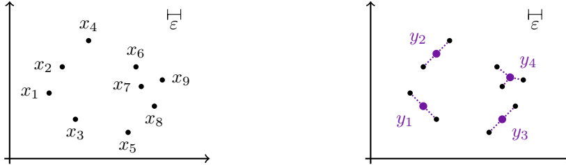
Figure 6.2: Example instance for uniform point cover (UPC, Problem 6.17). Left: nine source points x_1, \dots, x_9 . Right: a (4, \varepsilon) -cover y_1, \dots, y_4 .
